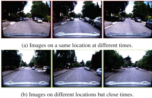
Figure 7: Images of the RobotCar dataset to show limited appearance distinction with dynamic changes on a same location and perceptual aliasing among different locations.
