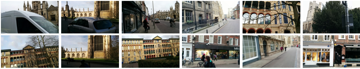
Fig. 11: Images with the largest uncertainty values and largest localization errors. All of these images contain one of the following situations causing difficult and uncertain localization: strong occlusion from vehicles, pedestrians or other objects, motion blur, are taken from an area at the edge of the scene or are distant from a training example.
