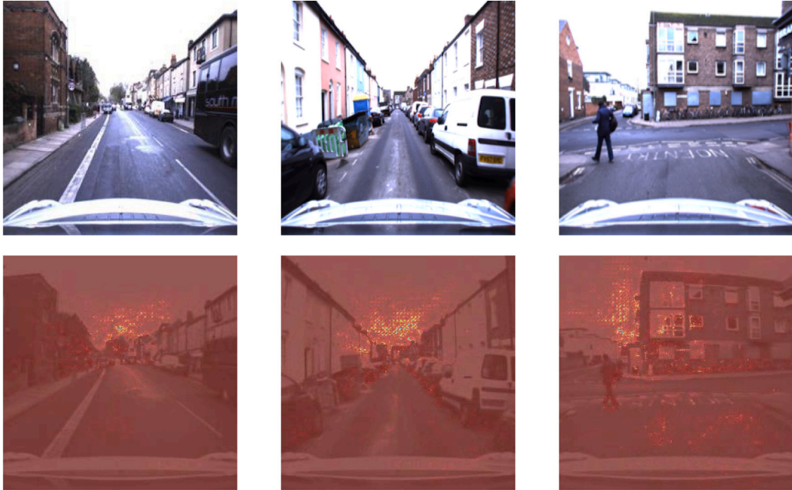
Fig. 9. Heatmap visualization of attention weights from Oxford RobotCar generated from the original image (top) and with attention model (bottom). TransBoNet learns to ignore visually uninformative features, such as roads in the above figure, and instead focus on more unique objects, such as distant skylines. It also learns to reject some dynamic objects, such as vehicles in the middle figure and pedestrians in the bottom figure, so as to achieve more robust camera localization.
